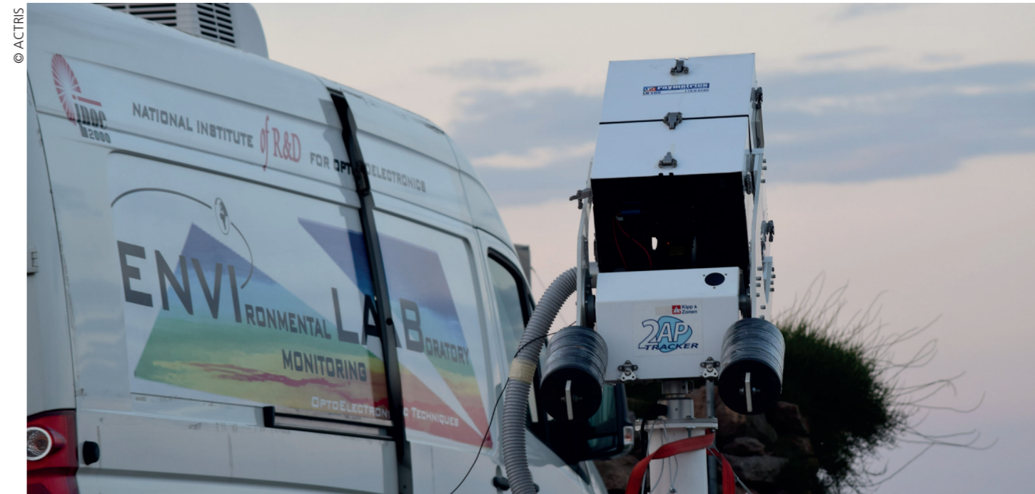
Mobile laboratory for atmospheric measurements during Pre-Tect campaign in Crete, Apr. 2017 – daytime observations of marine aerosols and clouds with the scanning UV polarization lidar
